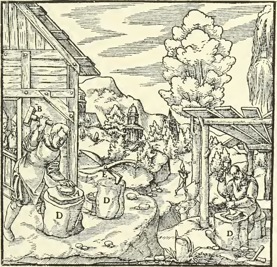
A—MASSES OF METAL. B—HAMMER. C—CHISEL. D—TREE STUMPS. E—IRON TOOL SIMILAR TO A PAIR OF SHEARS.
